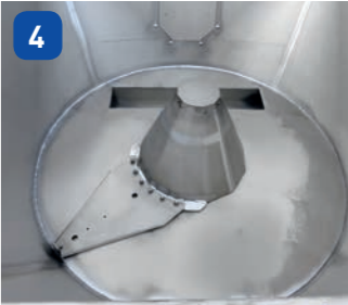
Dosing blade The continuous rotation of the stainless steel dosing blade prevents the substrate from bridging above the screw out-feed. The blade, which is equipped with a plastic slider bearing, processes the material such that it can be further processed by the subsequent screw technology. The revolution speed of the blade socket is set to the exact conveyor capacity of the base frame screw. Due to the flat design of the blade, minimal driving power is required. This also makes it very insensitive to foreign bodies. The dosing blade can easily be replaced during inspection.
