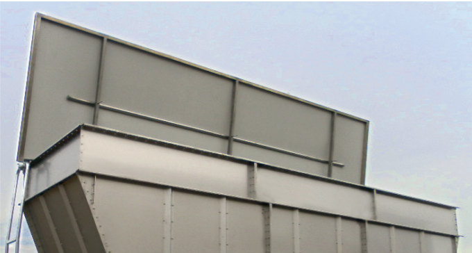
Cover In order to reduce emissions and weathering, the solid matter dosing unit can be equipped with a hydraulically operated cover. The cover consists of a stainless steel frame covered with a UV-resistant tarp. The cover can be operated via radio remote control upon request.
