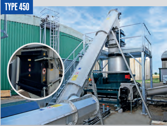
A two-part screw conveyor system consisting of a TYPE 450 horizontal and an inclined screw conveyor with magnetic separator transfers the substrate to a vertical shredder.
