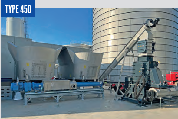
Two independent feed systems feed two liquid feed systems. One of them feeds into a vertical shredder via a two-part TYPE 450 screw conveyor system with magnetic separator. It is then transported to an external liquid feed system by a TYPE 450 flex transfer. The other is equipped with a TYP 450 horizontal screw conveyor with flexible transfer that conveys into an external liquid feed system.
