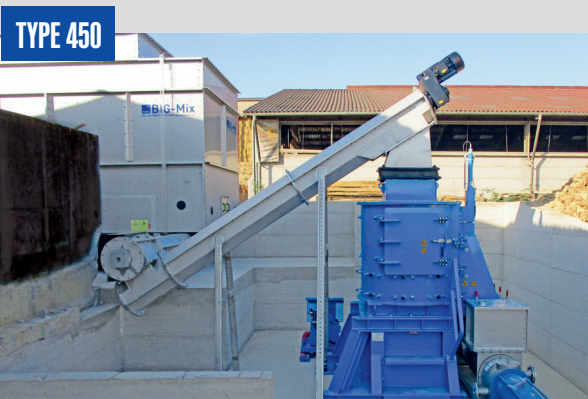
A two-part TYPE 450 screw conveyor system consisting of a horizontal and an inclined screw conveyor feeds a vertical shredder. The feed rate is individually adapted to the performance level of the downstream vertical shredder and the desired degree of shredding.
